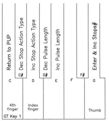
Use key 3 to toggle between SAMs and LEDs. If you have selected SAMs, use key 5 to select the pulse length, any number between 5 and 12 scan cycles, 8 being a good medium choice or starting point.
