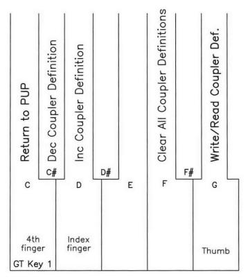
Use key 3 to increment the coupler definition, and key 2 to decrement this definition. Turn on the appropriate coupler to program this selected definition into the input pin's memory. The LCD will go blank and increment to the next definition when the coupler is turned off.
