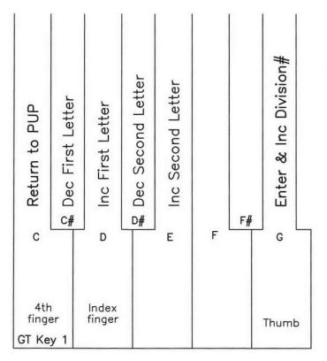
With 'enter' key 8, accept this default and the LCD will increment to the next division number if assigned in 1. Input Card Address Assignments. If Division 2, then PD will be displayed, also a default name that cannot be changed. With key 8, enter this default and the LCD will increment to the next assigned division number. Displayed will be two upper case letters that are stored in memory for this division. If programming from scratch, "AA" will be displayed.
